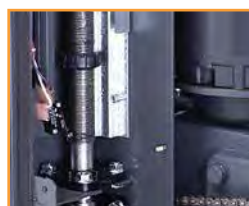
limit switches direct driven and easily adjustable
