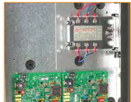
solid state motor control no relay contacts to wear out or burn
