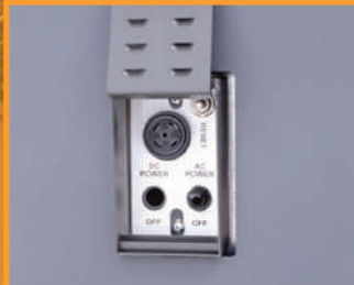
Built In power switch and reset switch
