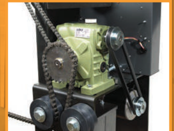
Full Size Gearbox heavy-duty 30:1 ratio gearbox
